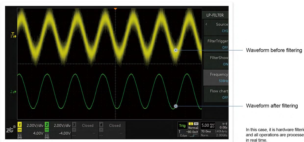
In this case, it is hardware filtering and all operations are processed in real time.
