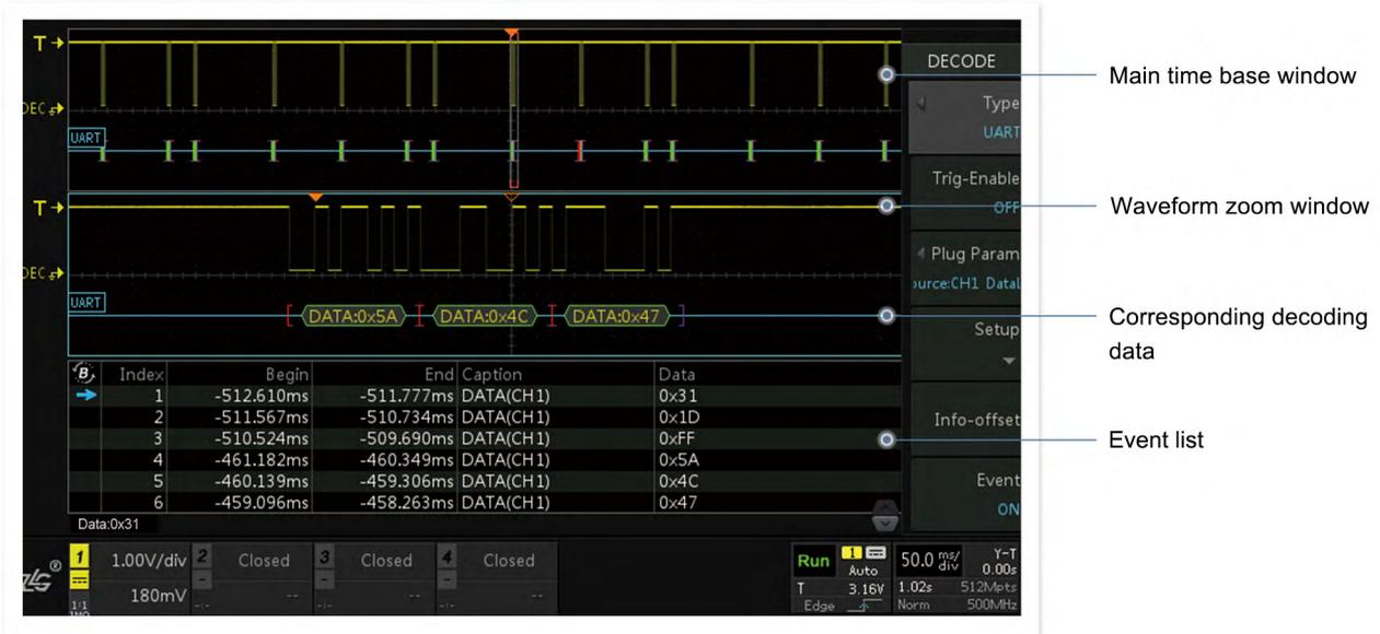
Supported protocol decoding types: UART, SPI, I2C, USB, PS/2, DALI, Wiegand, 1-Wire, DS18B20, HDQ, SD-SPI, SD-SD, IrDA, Manchester, DiffManche, Miller, DHT11, SHT11, NEC, RC5, RC6, CAN, LIN, FlexRay, CAN FD, MVB, ISO7816, Modbus, WTB, MIL-STD-1553B, and MIPI-DSI.
