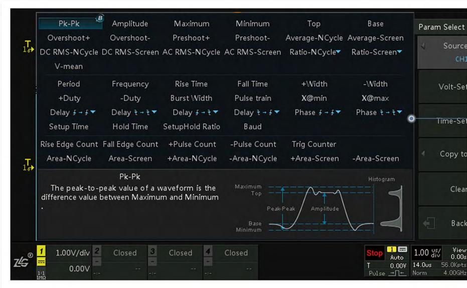
Supports measurement of **51** parameters
