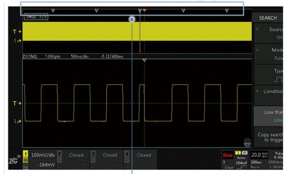
All signals conforming to the conditions will have a white inverted triangle.
