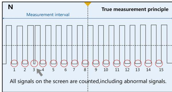
For data mining oscilloscopes, all periodic signals can be measured, realizing true measurement.
