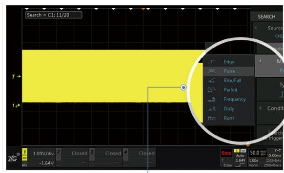
Set the search conditions, such as edge, pulse width, runt, rising/falling time, cycle/frequency, etc.
