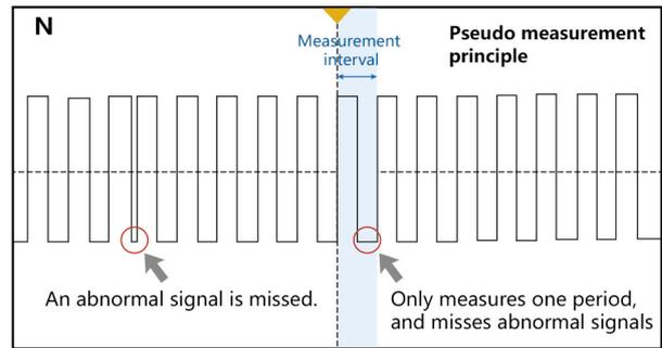
For traditional oscilloscopes, only one periodic waveform is measured near the triggering position, which is a pseudo measurement.
