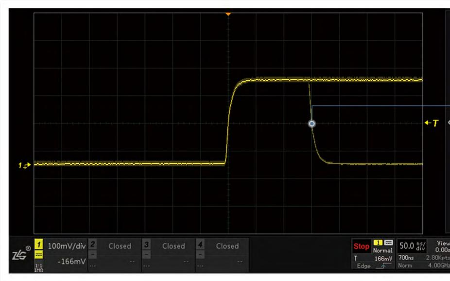
Only oscilloscopes with a **high capture rate** can capture abnormal signals with **low probability of occurrence**.
