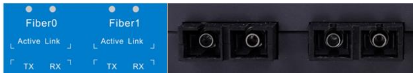
Figure 2.7 Optical fiber interface and indicators
